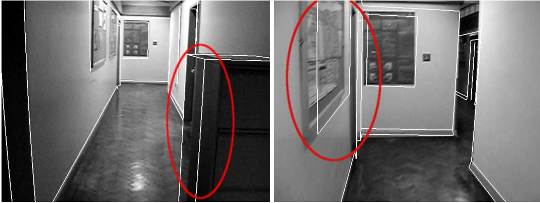
Figure 4.1: Two examples of a single hypothesis edge tracking system ‘locking’ on to an incorrect edge and falling into a local minimum.
