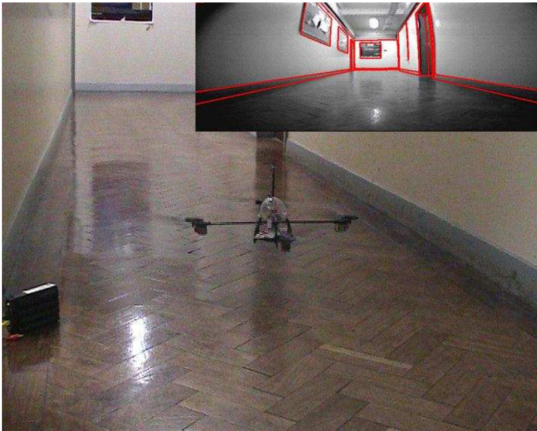
Figure 7.13: The helicopter automatically flying along a corridor and an insert showing the tracked image from the onboard camera.
