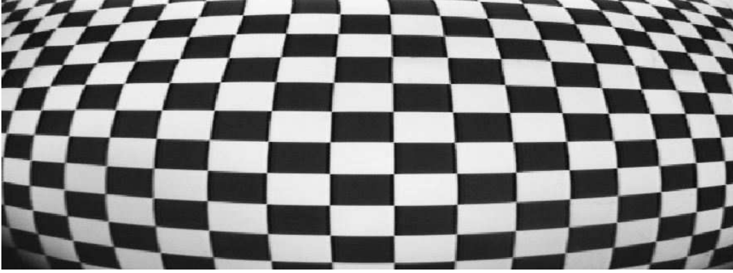
Figure 3.5: A view of a calibration grid seen through the MAV camera, showing significant barrel distortion.
